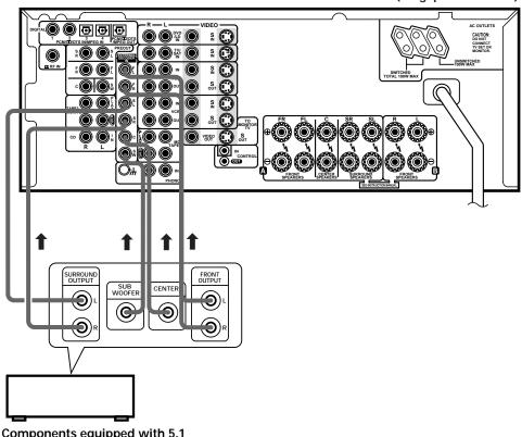
Components equipped with 5.1 channel analog output jacks
